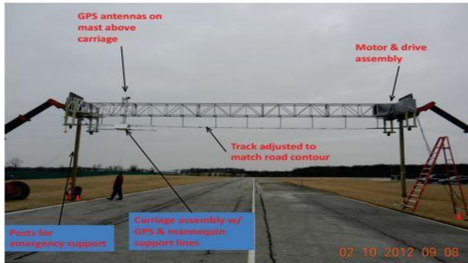
Figure 1: Outdoor mannequin utilizing overhead gantry (Carpenter, M. G., et.al., 2013)
